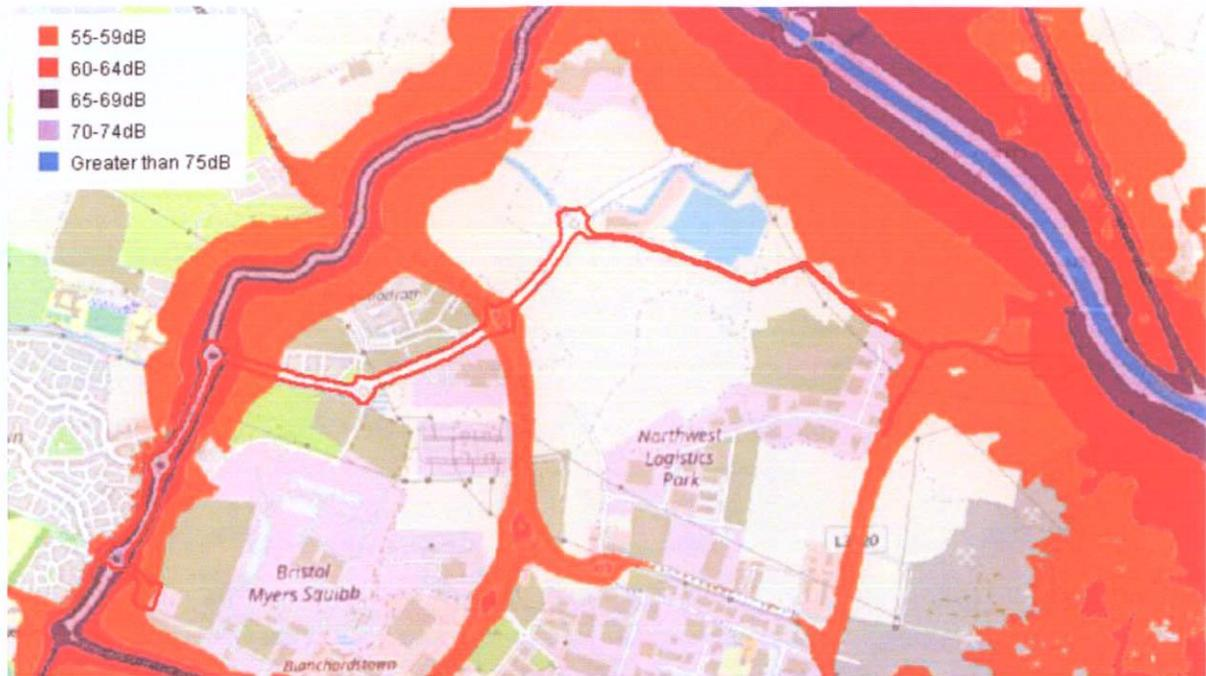
**Figure 7.3** L<sub>den</sub> contours for road traffic noise
