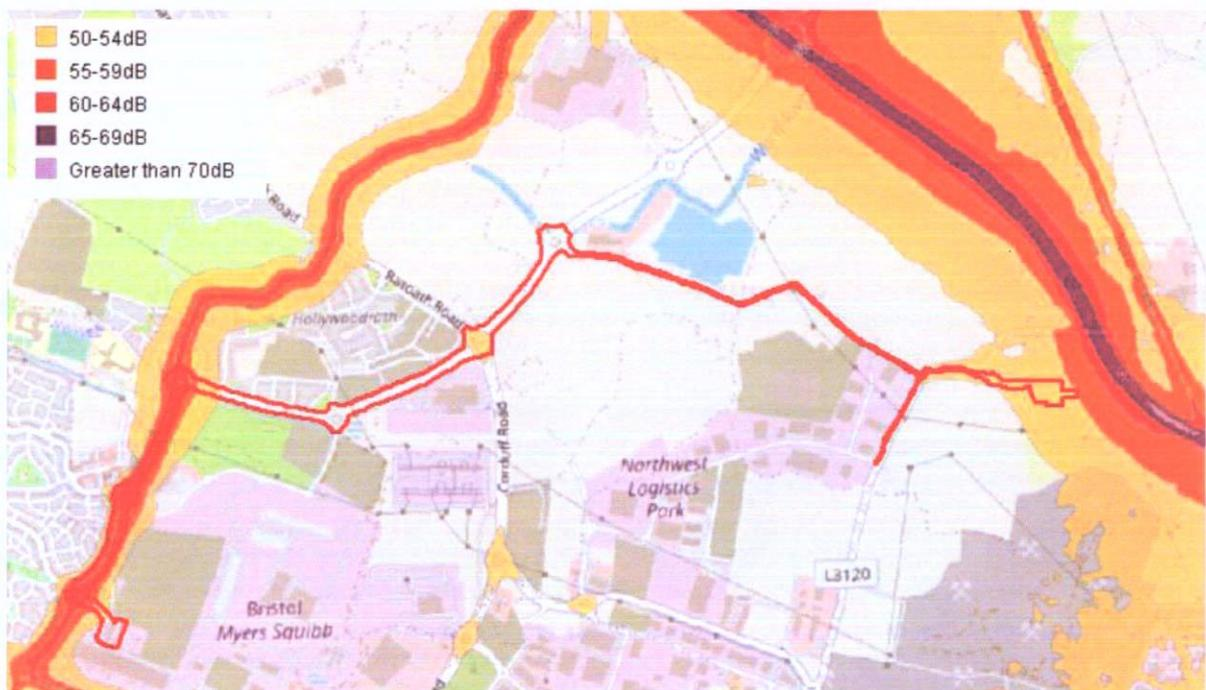
**Figure 7.4** L<sub>night</sub> contours for road traffic noise
